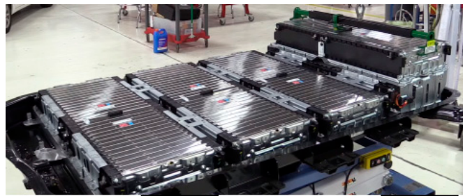
Figure 9. Chevy Bolt battery with cooling metal plates on the surface of battery cells.
