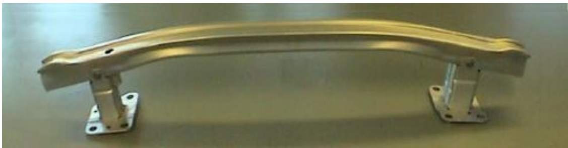
Fig. 6-38: Extruded bumper beam with crash boxes [GIL04]
