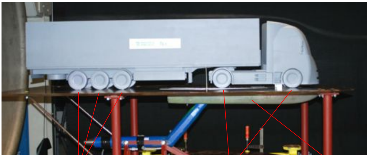
Fig. 6-26: Hardware models for wind tunnel tests
