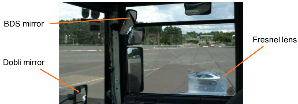
Fig. 4-14: Supplementary devices to reduce blind spots [DOD09]
