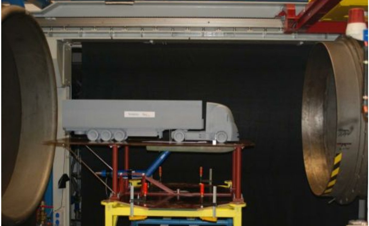
Fig. 6-26: Hardware models for wind tunnel tests
