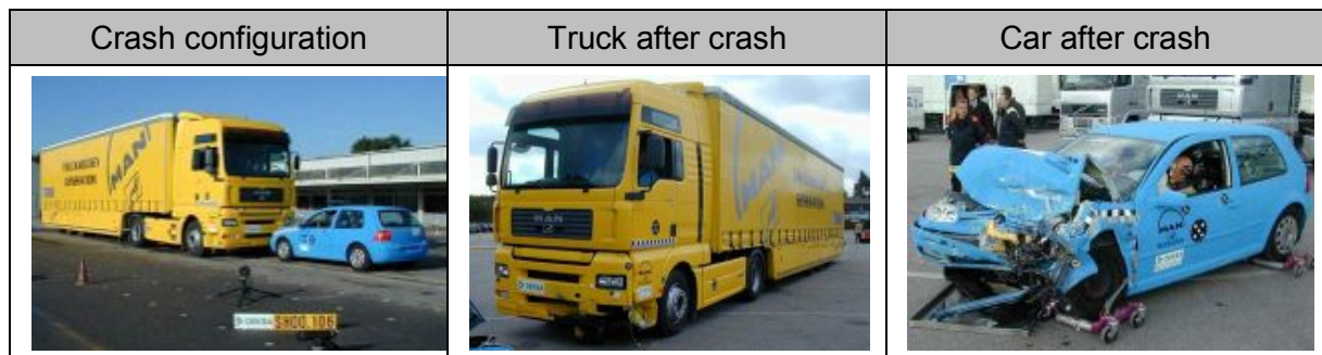
Fig. 6-50: DEKRA truck against car crash test [DEK10]
