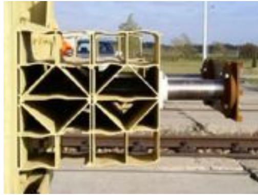
Fig. 6-40: “Safetram” system for trains [GIL04]
