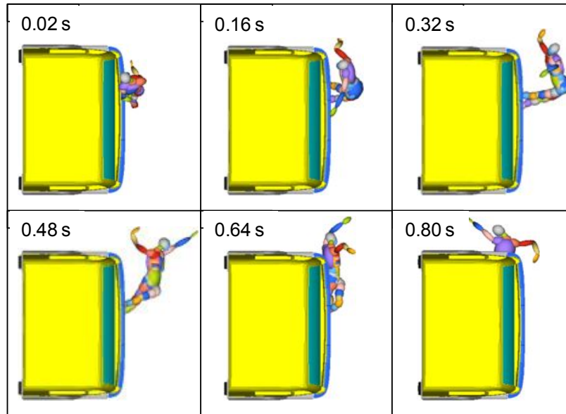
Fig. 6-56: Kinematics of the 50 % male in the straight forward driving situation [FAS08]
