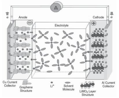
Figure 3: The structure of a lithium-ion battery cell
